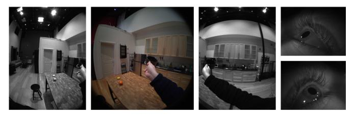
Figure 2. Example images from the Project Aria device cameras. Left to right: left Mono Scene camera, POV (RGB) camera, right Mono Scene camera, two Eye-tracking cameras. Output of POV (RGB) and Mono Scene cameras are rotated for visualization.
