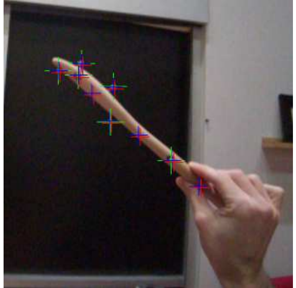
Figure 9: Cropped version of example Aria image used for system accuracy tests with results. Red: system's estimate of where the markers should project. Green: hand labels of where the markers are located in the image. Blue: system estimate of where the markers should be after optimizing for the true object relative pose.
