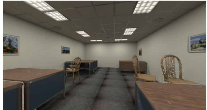
Figure 18: Mesh reconstruction of the first synthetic dataset. Note that the rough triangulation of parts of the chairs is due to a poor viewing angle throughout the sequence.
