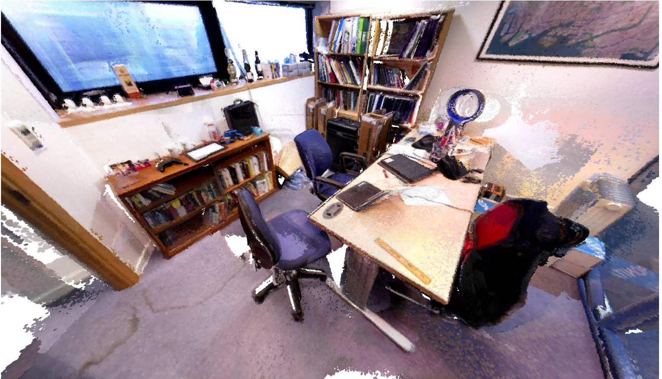
Figure 1: Comprehensive scan of an office containing over 4.5 million surfels captured in real-time.
